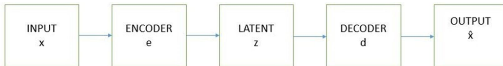
Fig. 5: Block diagram for the Variational Autoencoder (VAE).
