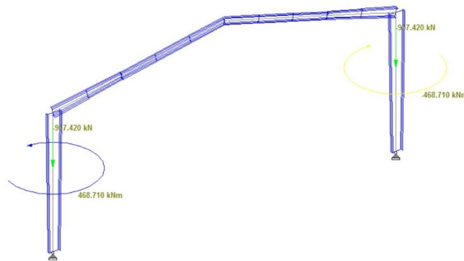
Fig. 11: Factored load and couple moment acting on supporting columns of pre-engineered steel frame
