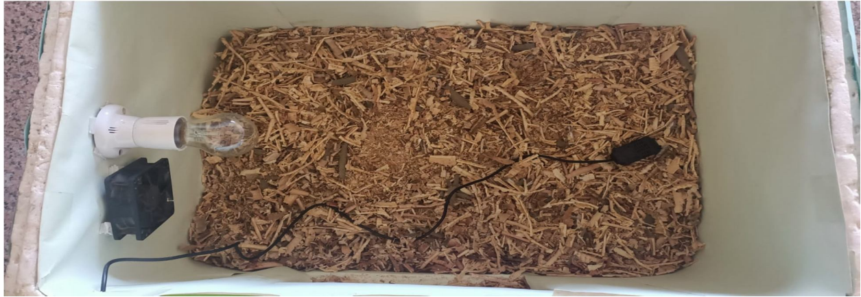
Figure 2.1. The egg brooding unit made and over all circuits established for efficient working.
