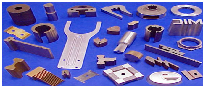
Fig. 4: Components manufactured by WEDM
