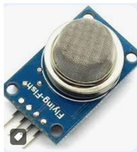
Fig.5 Gas Sensor Module
