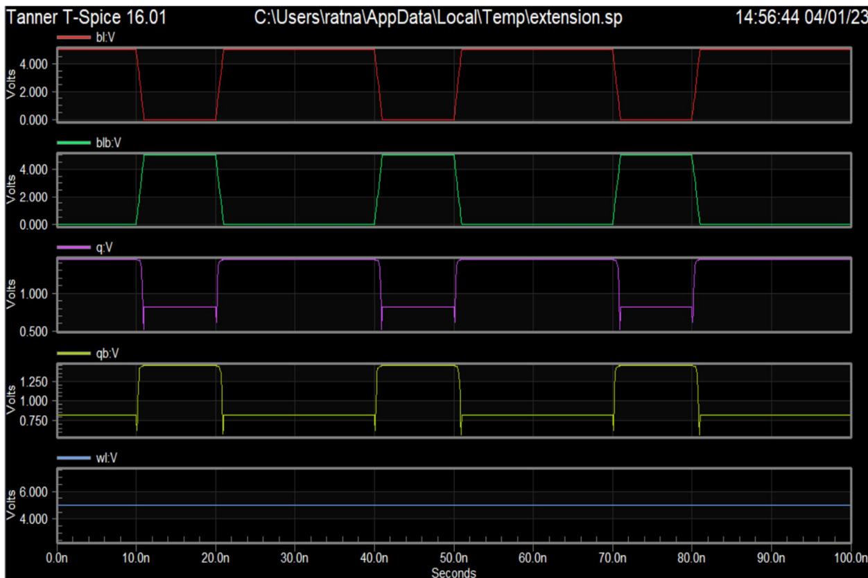
Fig: Transient response of 10T SRAM Cell
