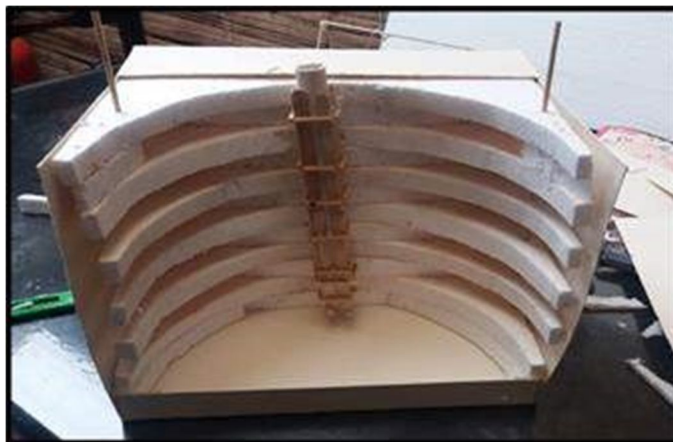
Fig. -5: Prototype of the covering made for the sensors. Canadian Biohogar well, 2021 Source: SIE2
