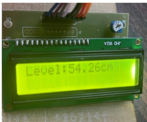
Figure 5: LCD Display of garbage level monitoring
