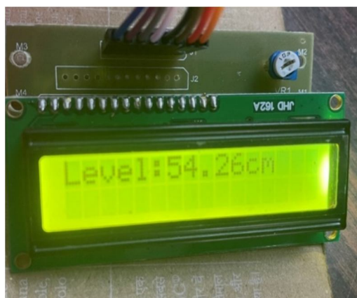
Figure 5: LCD Display of garbage level monitoring
