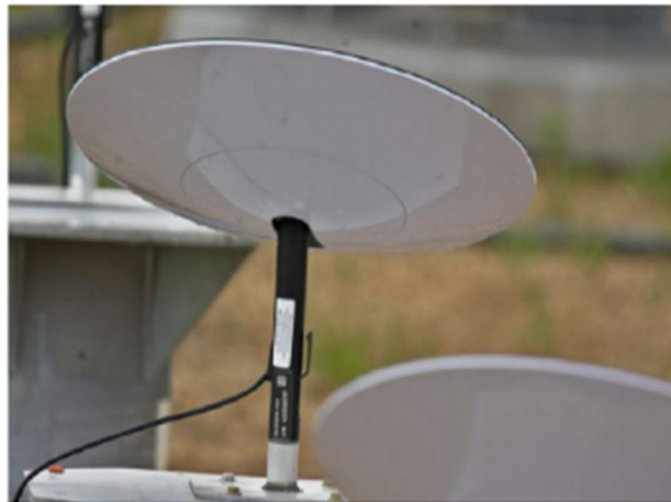
Figure-4: Showing the Image of Tracker Antenna to track the signals from Starlink Satellite
