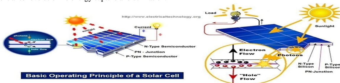
Fig 1: Operating principle of solar panel
