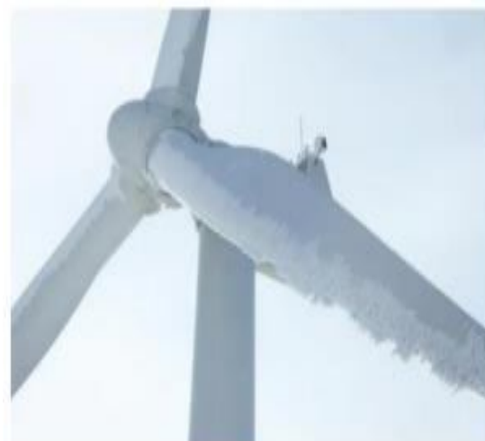
Figure 7: Icing on the wind turbine.
