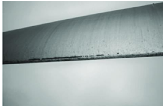
Figure 8: delamination of blade.
