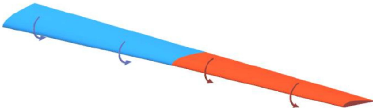
Fig.3 Two-piece blade concept of PLTC
