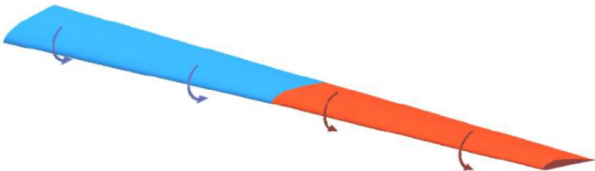
Fig.3 Two-piece blade concept of PLTC
