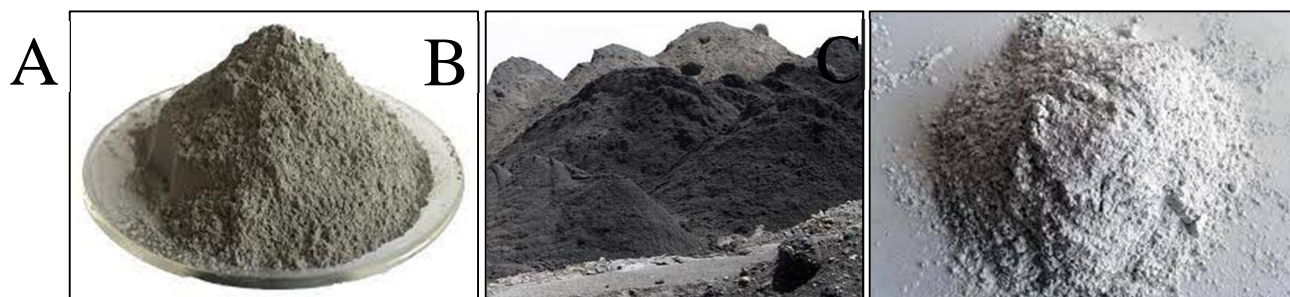
Fig. 1 Material used for Soil Stabilisation (a) Silica Fume (b) Fly Ash (c) GGBS
