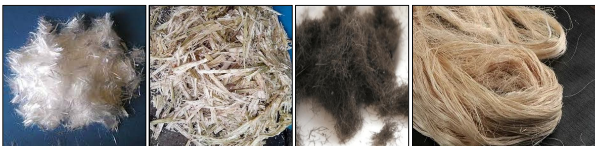
Fig. 2 Material used for Soil Stabilisation (a) Polypropylene fiber (b) Sugarcane bagasse (c) Human hair fibers (d) Banana fiber
