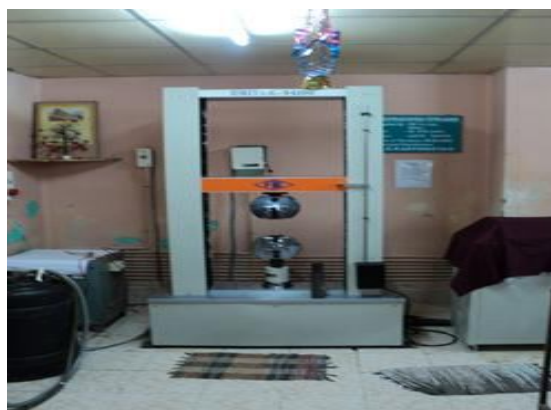
Fig-5: Compression testing machine (UTM)
