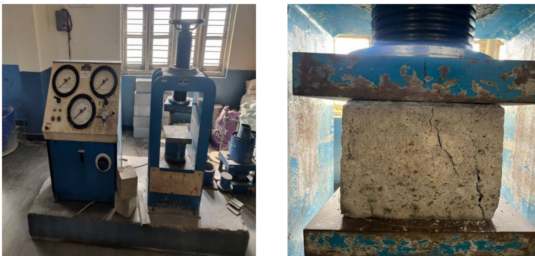
Figure 4.7: Compressive Testing Machine
