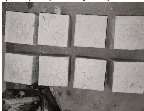
Figure 4.6: MOC concrete cubes exposed to air
