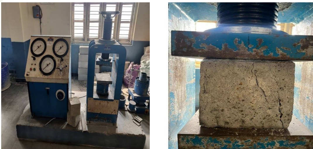
Figure 4.7: Compressive Testing Machine
