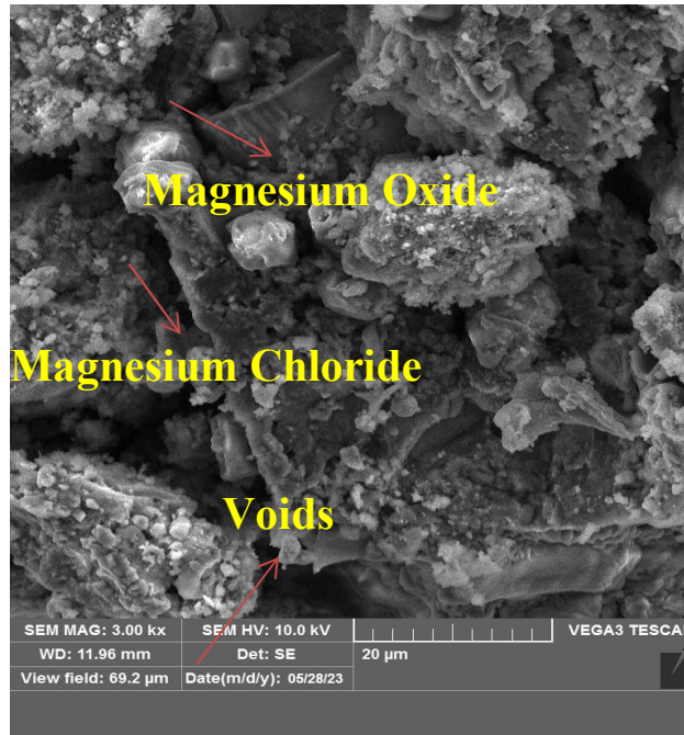
Figure 6.2: Shows the internal structure of MOC concrete that has been heated 150°C using MgO
