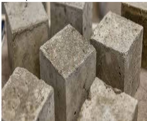
Figure 4.2: OPC concrete cubes
