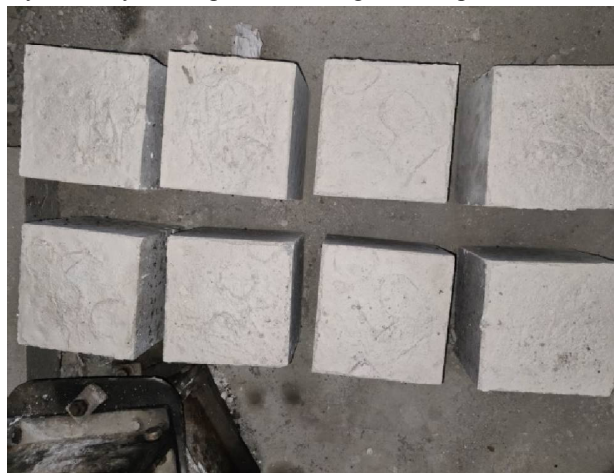
Figure 4.6: MOC concrete cubes exposed to air
