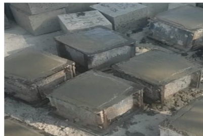
Figure no 4 :Cube Test (150x150x150) mm.
