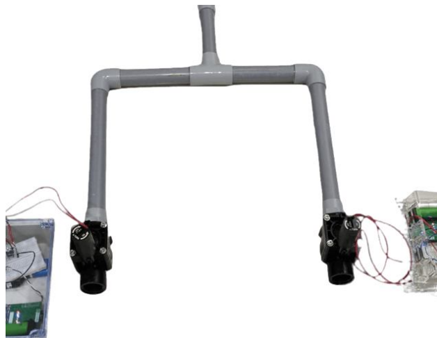
Fig. 3 Valve Setup of the System
