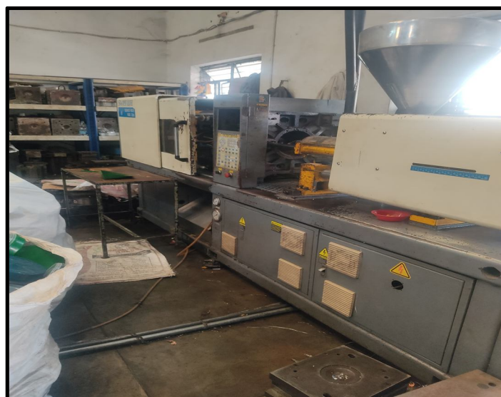
Fig 4:A image of plastic injection molding machine
