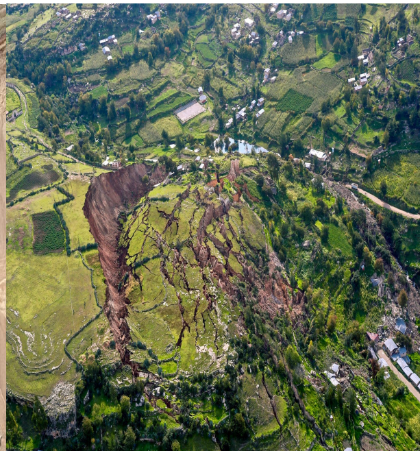
Fig. 6b. Sliding Planes near Cusco, Peru in 2018 Top Right) used to Form a Single Continuous Line, but have been Split Apart by Movement along the Fault
