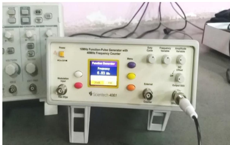
Figure 6 Function generator to generate desired Sine Wave
