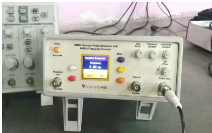
Figure 6 Function generator to generate desired Sine Wave
