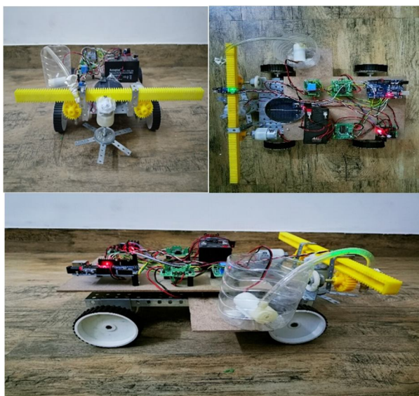
Figure 6: Weed Cutting and Pesticide Spraying Agbot
