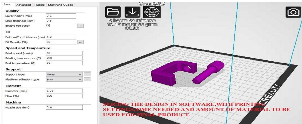
Fig. 2 – Making the design ready for slicing with few printable settings ,time needed and amount of material to beused.
