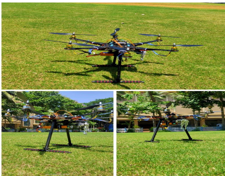
Figure 2: Proposed system for fire extinguishing UAV.
