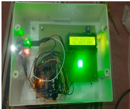
Figure 3: Integrated Fire and Gas Detection System
