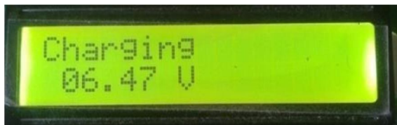
Fig. 4. LCD shows receiving voltage
