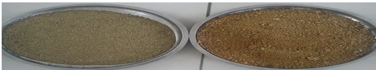
Iron Ore Slickens Natural Sand Figure 1: Comparison between natural sand and Iron Ore Slickens
