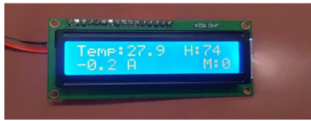
Figure 2. Temperature, Humidity, Current and motor readings from LCD display
