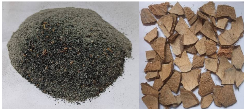
Fig. 1 Agro-Waste used in concrete (a) RHA and (b) CS
