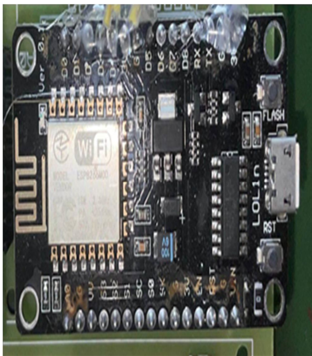
FIG 7 : ESP8266 Node MCU WiFi Development Board
