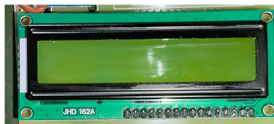
FIG 6 : LCD (LIQUID CRYSTAL DISPLAY)
