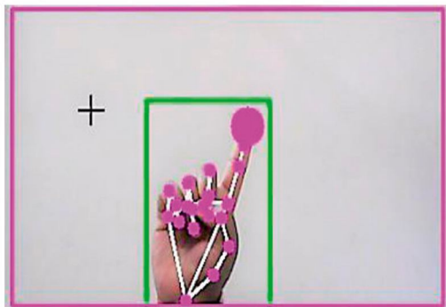
Figure 4. Detection of which finger is up.
