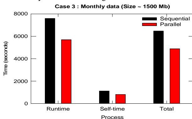
Fig.6.1 Time Taken to Process Monthly Data in Sequential (Black Colour) and Parallel (Red)
