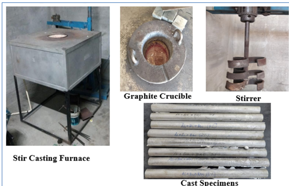
Fig 4.4 Stir Casting Process
