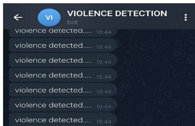
Fig 6: Alert message via telegram for violence detection
