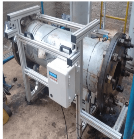
Fig. 3 Images of the apparatus used for the paraffin deposition production with the coupons.
