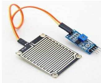
Fig. 5.KG004 Rain Drop Sensor
