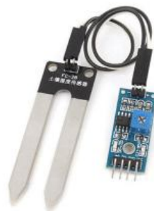
Fig. 3.FC-28 Soil Moisture Sensor
