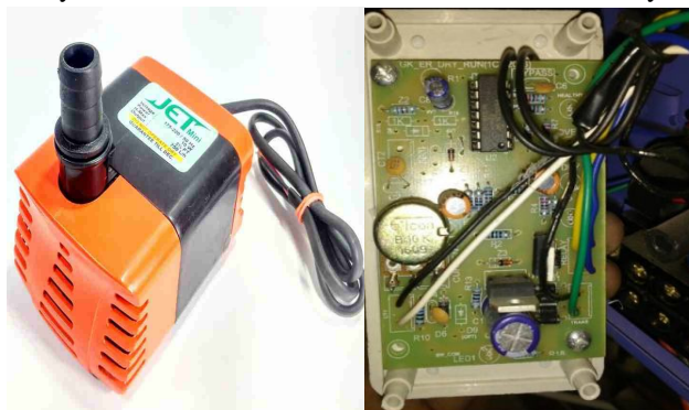
Fig. 6. Submersible Water Pump with Controller
