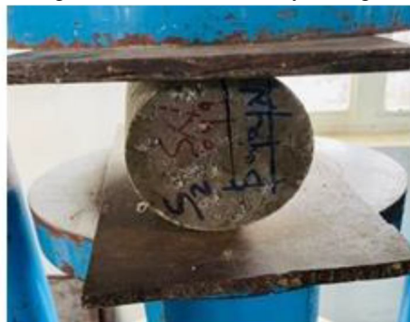
Fig5. Split tensile test
