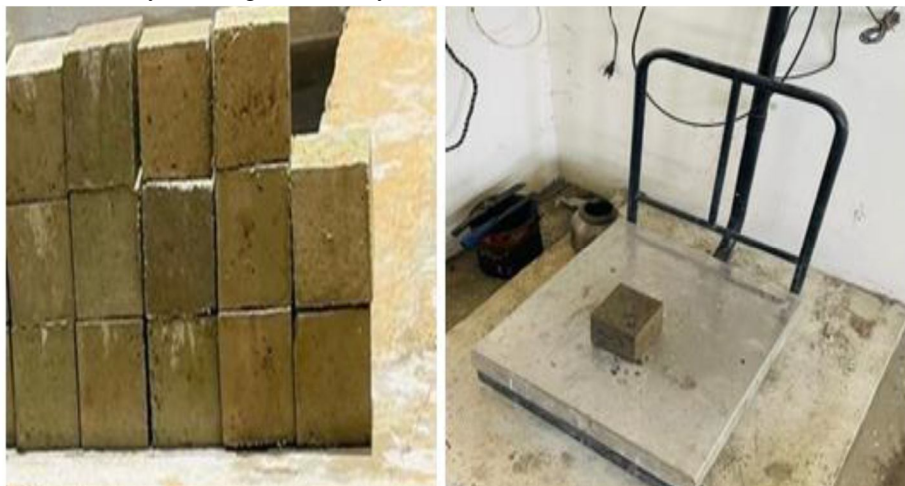
Fig 6. Water absorption test
