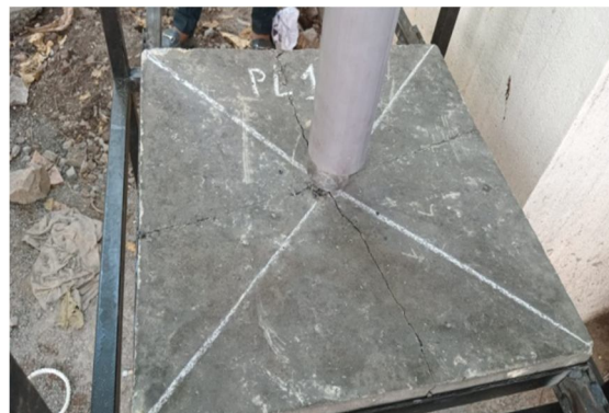
Photographs of Cracking Pattern Seen on Impact Testing of Plates
