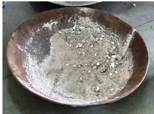
Fig. 1: Ceramic tiled aggregates broken pieces.
