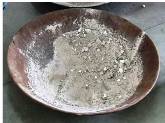
Fig. 1: Ceramic tiled aggregates broken pieces.
