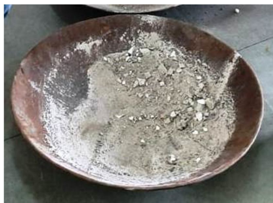
Fig. 1: Ceramic tiled aggregates broken pieces.
