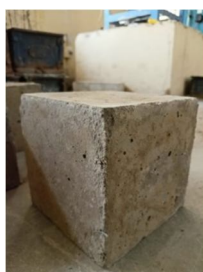
Fig:5 Specimen Of Cube
