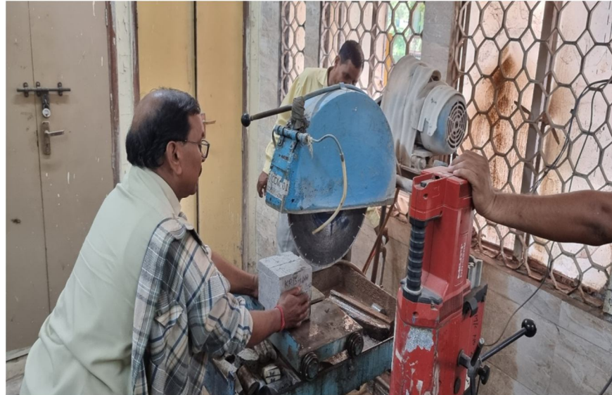
Fig. 4: Cutting of cubes
