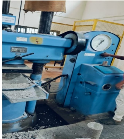
Fig 7. Split Tensile Strength Test
