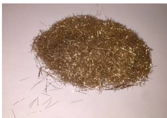
Fig 4: Brass coated Steel Fibres
