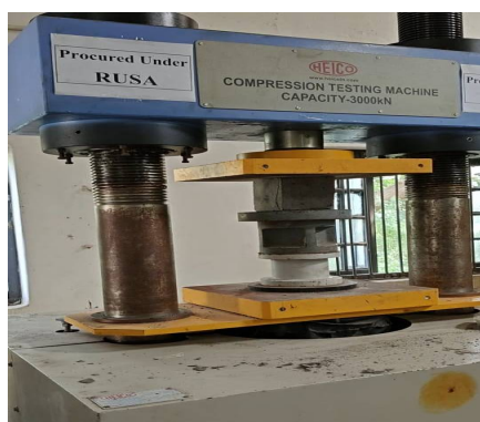
Figure 6. Performing Compressive strength test
