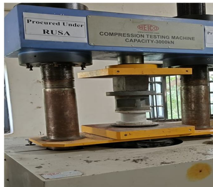
Figure 6. Performing Compressive strength test
