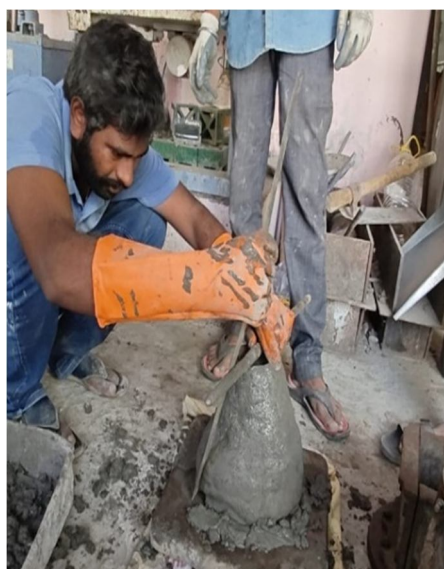
Figure 5 Performing Slump Cone Test
