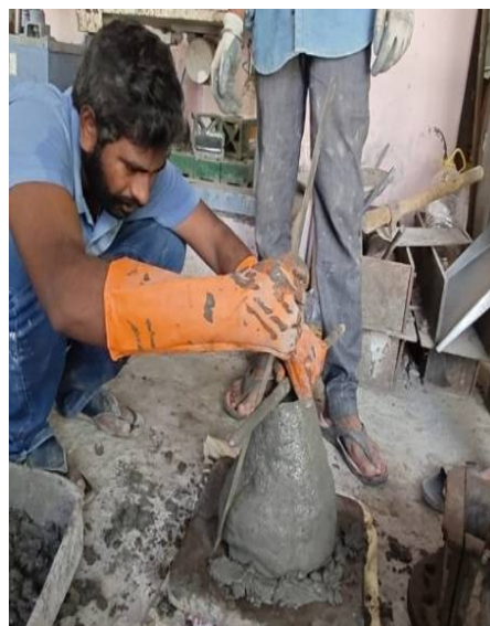
Figure 5 Performing Slump Cone Test
