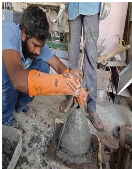
Figure 5 Performing Slump Cone Test
