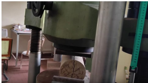
Fig 5 : Specimen after split test.
