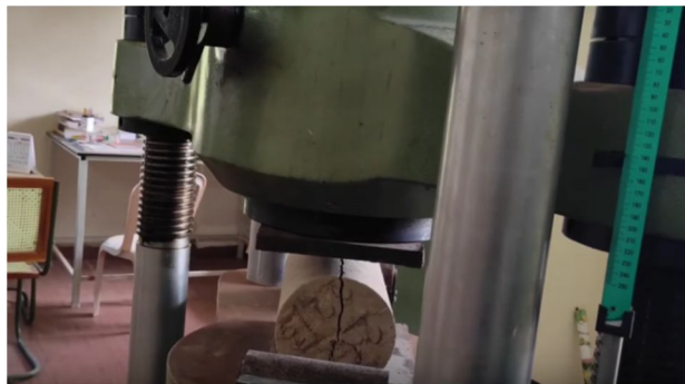
Fig 5 : Specimen after split test.
