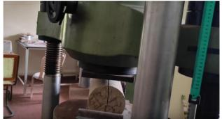
Fig 5 : Specimen after split test.
