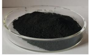
Fig 1: Graphene oxide powder.
