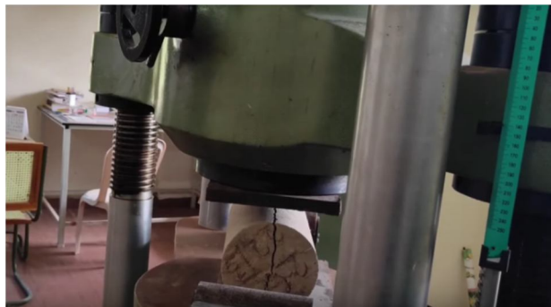
Fig 5 : Specimen after split test.
