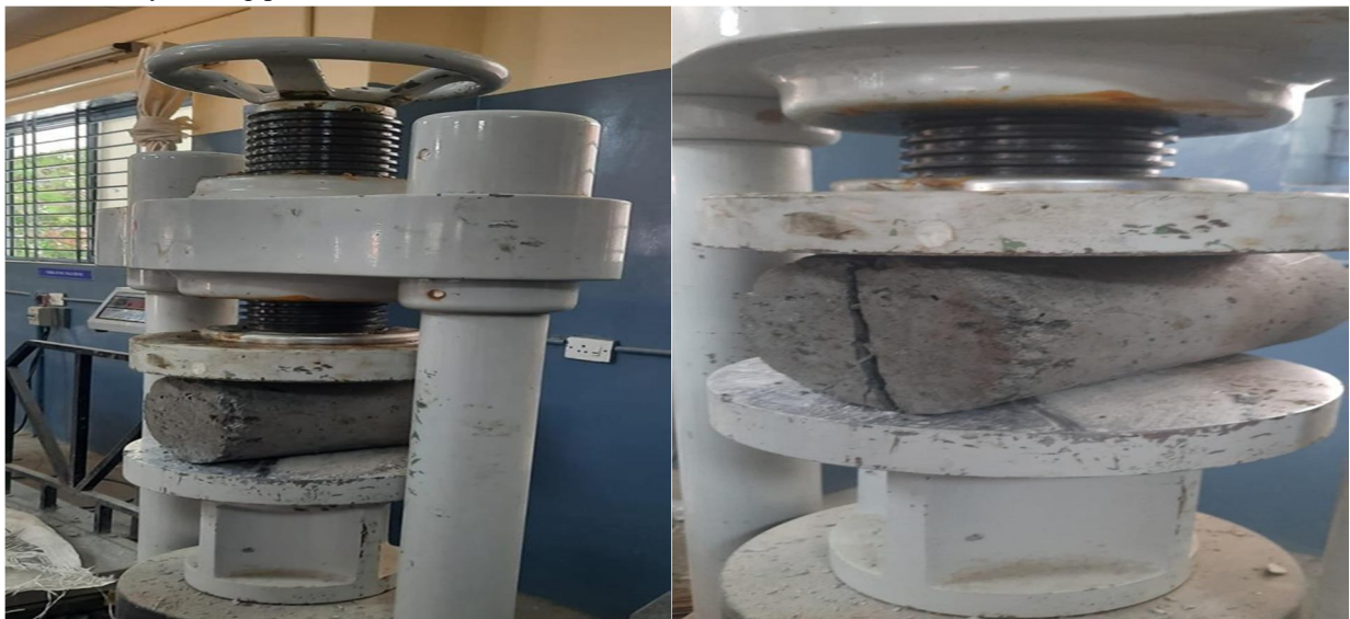
Fig 9: Split tensile strength test
