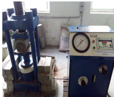
Split Tensile Strength Test on Cylinder
