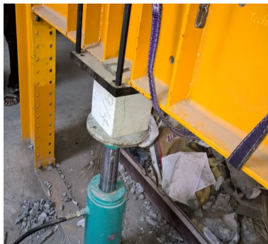
Compression Test on Cube
