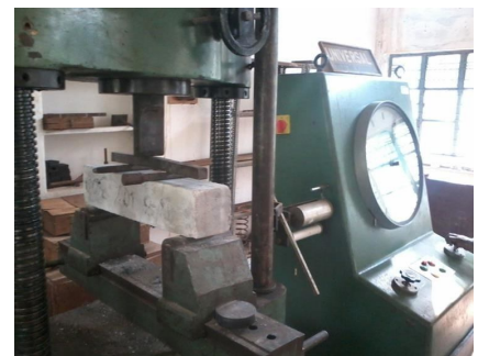
Flexural Strength Test on Beam
