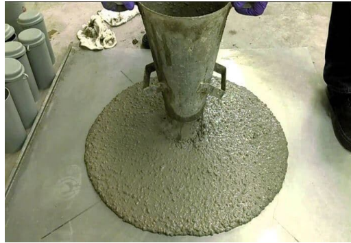
Slump Flow Test
