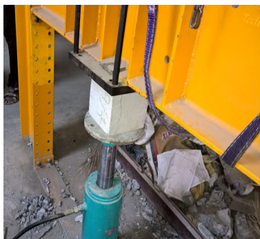
Compression Test on Cube
