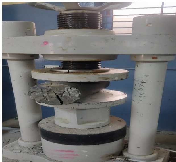
Fig 12 Split Tensile Test
