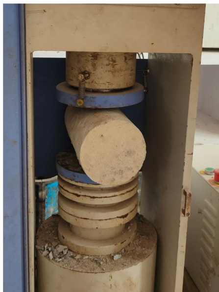
Fig 13, 14 Split Tensile Test & Graph of Split Tensile Test
