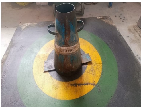
Fig 3,4 Slump Flow Test & Graph of Slump Flow Test(mm)
