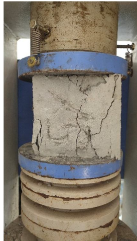
Fig 11,12 Compressive Test & Graph of Compressive Test
