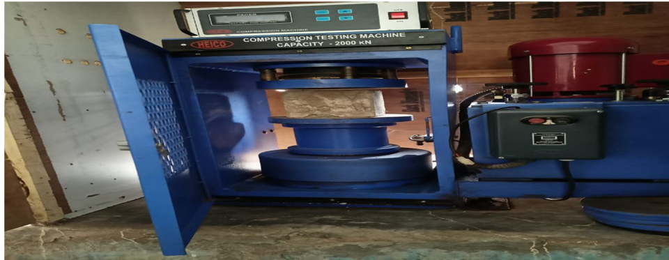
Figure no.1 Compressive strength testing
