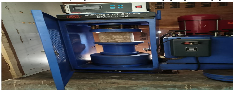
Figure no.1 Compressive strength testing
