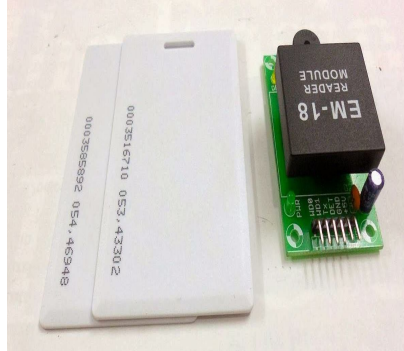
Fig.6; RFID Reader Module and tag
