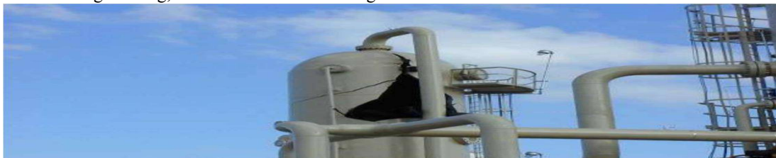
Fig. 2. Failure of pressure vessel during hydro Test.
