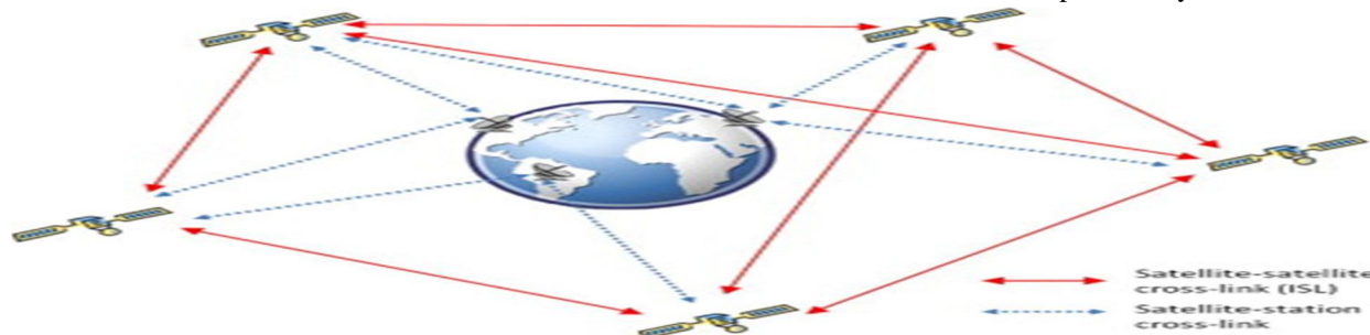
Fig.5 Inter-satellite communication and satellite-station communication
