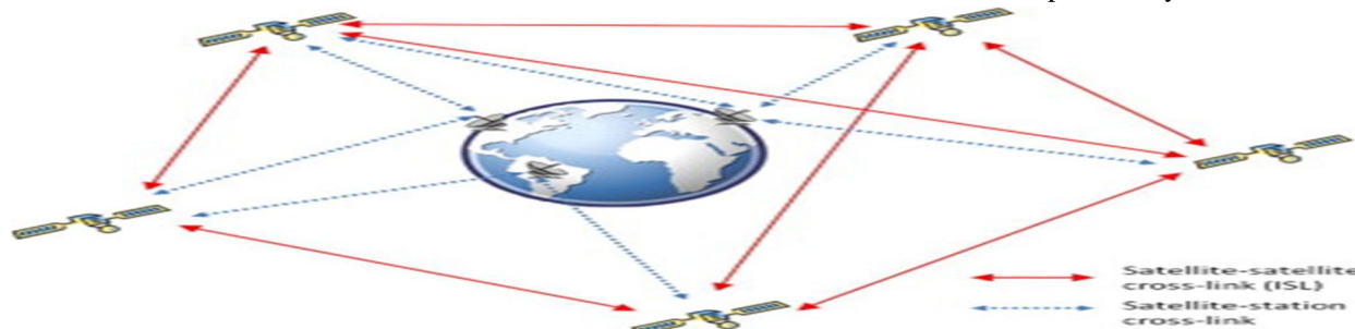
Fig.5 Inter-satellite communication and satellite-station communication
